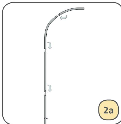
2. The flagpole sections have spring loaded bearings to help secure the parts together.
